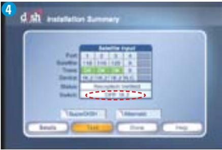
If the receiver shows a switch type of DPP1K.2, then a check switch test is not necessary. If it does not show a switch type of DPP1K.2, then make sure there are no checkmarks by "SuperDISH" or "Alternate," and select "Test."
