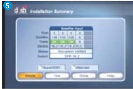
Verify that the check switch resulted in a switch type of DPP1K.2 and that there is a green 'OK' status on Satellite 110, 119, and 129.
